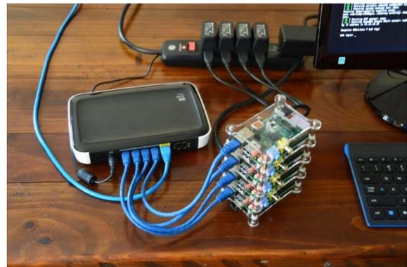
Figure 11. Raspberry Pi High-Performance Computer
