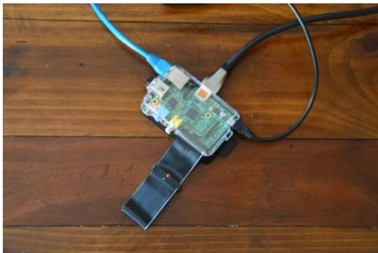
**Figure 5. Raspberry Pi with GPIO Cable and LED**
