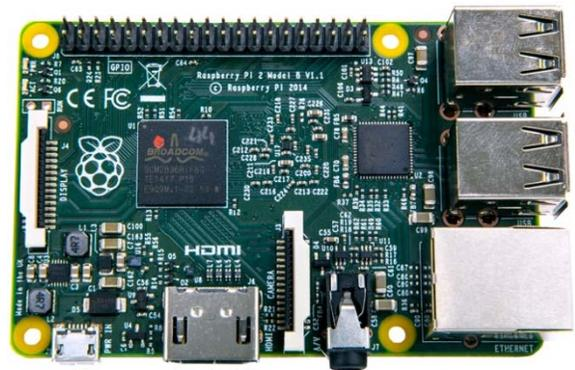
Figure 2. Raspberry Pi Model 2 Quad-Core 1024 MB
