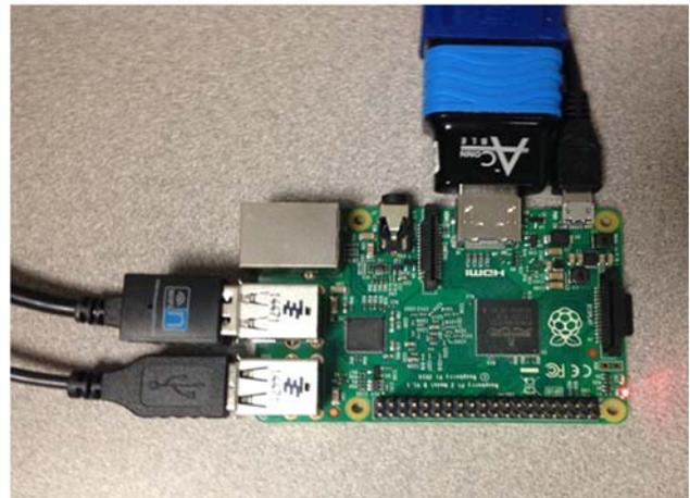
Figure 1. Raspberry Pi 2 Model B
